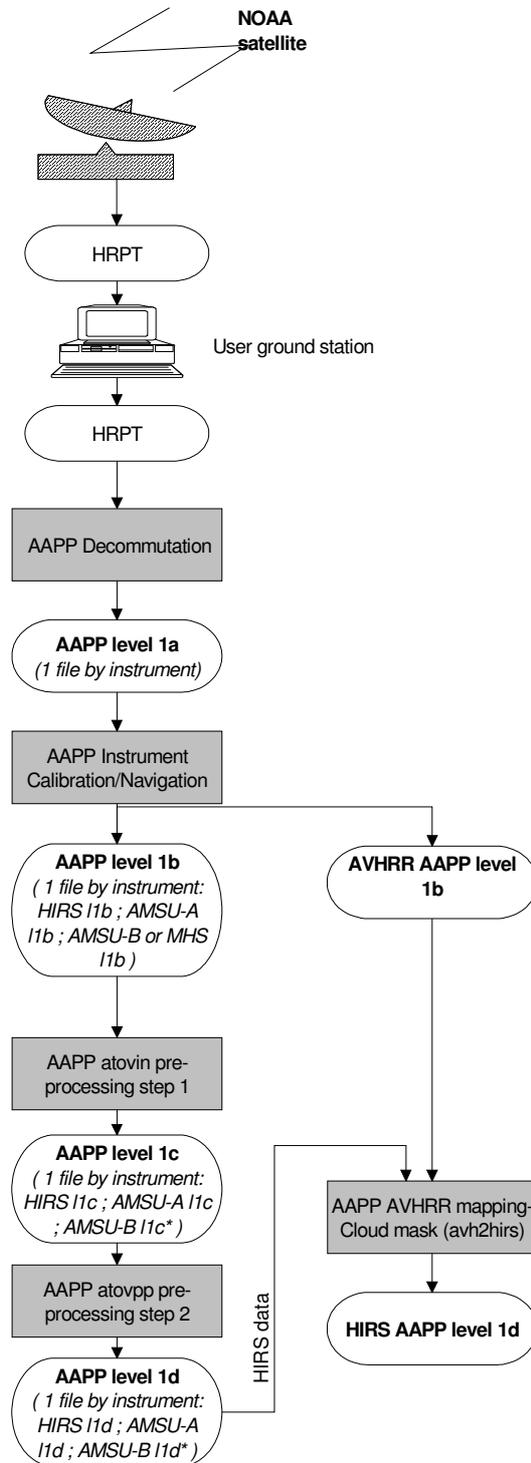
**Figure 2: AAPP processing chain for NOAA satellites.**
