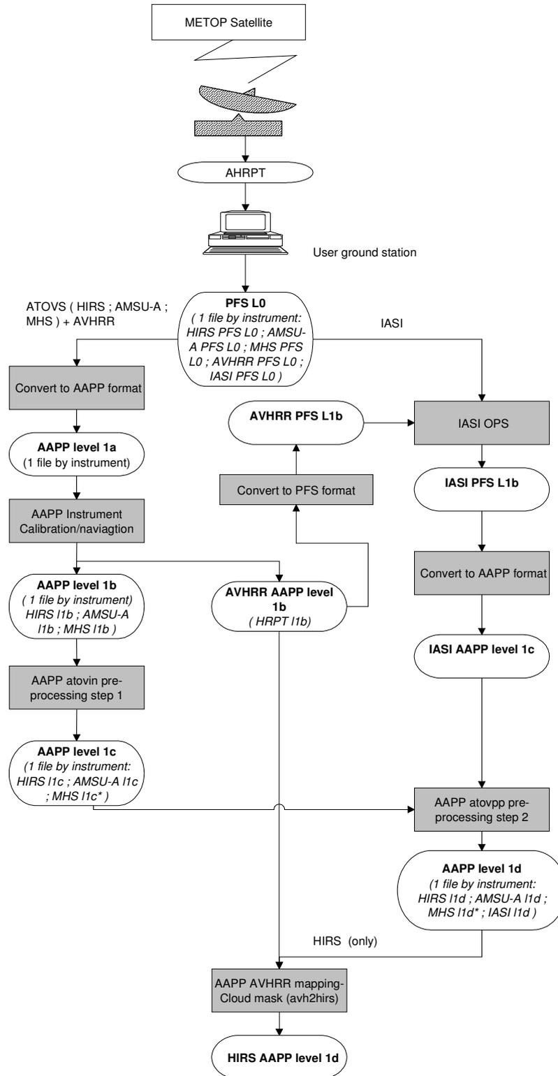
**Figure 3: AAPP processing chain for MetOp satellites.**
