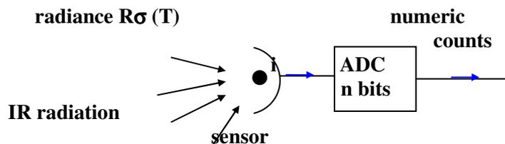
Figure 8: One IR channel for radiance measurements.
