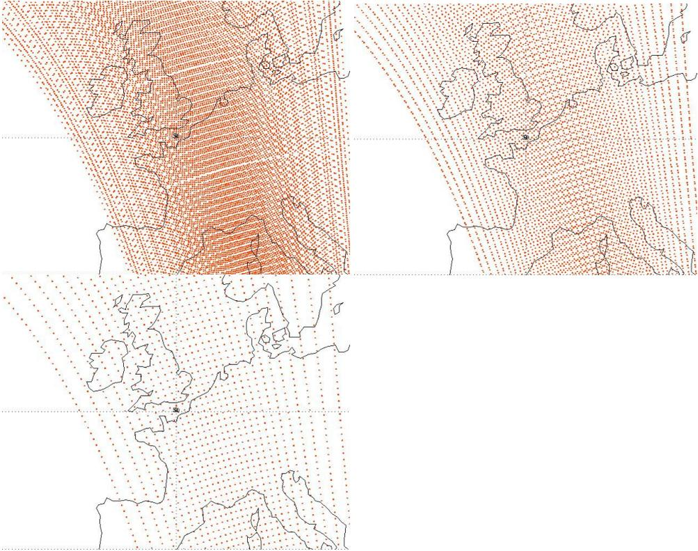
**Figure 10: Illustration of thinning options for CrIS: full resolution (9 detectors), 4 detectors, 1 detector.**
