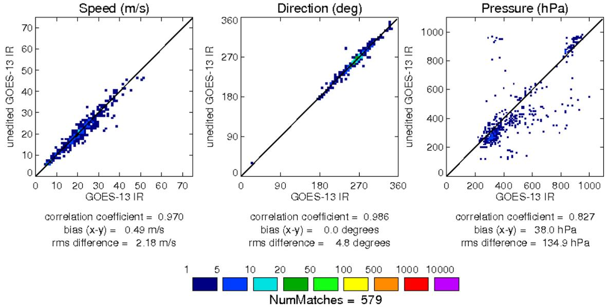
Figure 21: Speed, direction and pressure histograms for unedited heritage vs nested tracking GOES-13 infra-red AMVs. 9/3/17, 06Z cycle, co-located within 10km and 10 minutes, within a box 30-50° N, 50-75° W.
