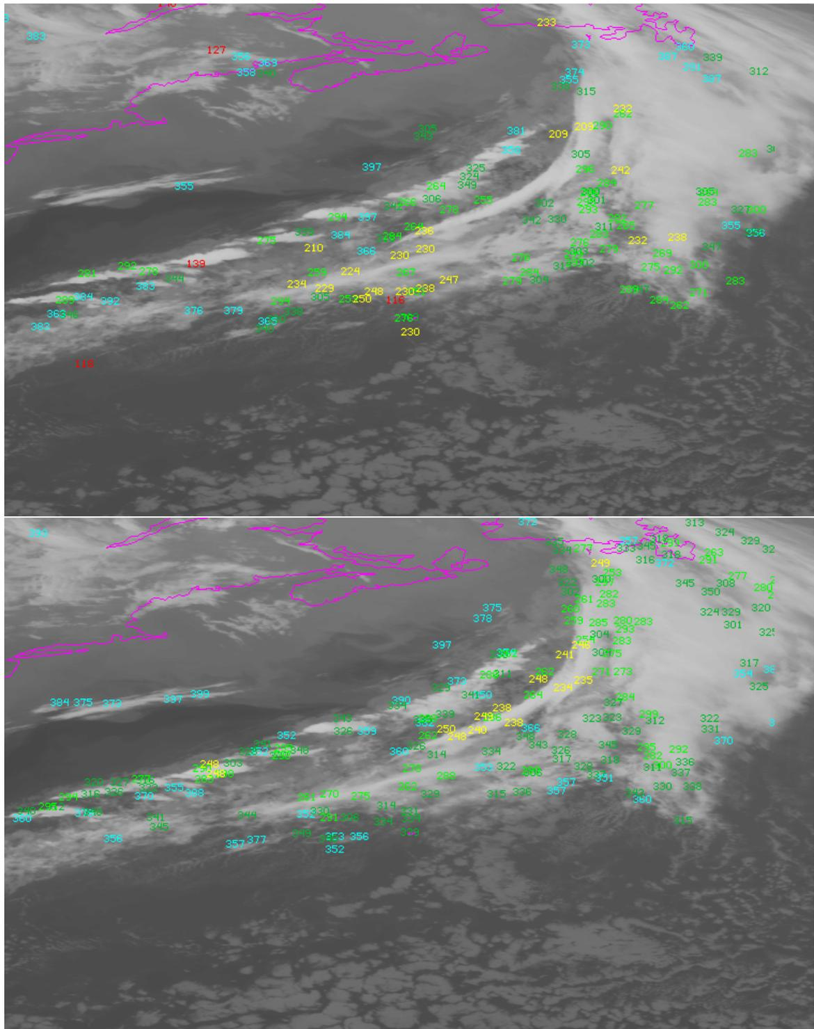
Figure 20: AMV pressures (hPa) of unedited heritage (top) and nested tracking (bottom) AMVs. Image shown is GOES-13 IR channel, at 0545 on 09/03/2017.
