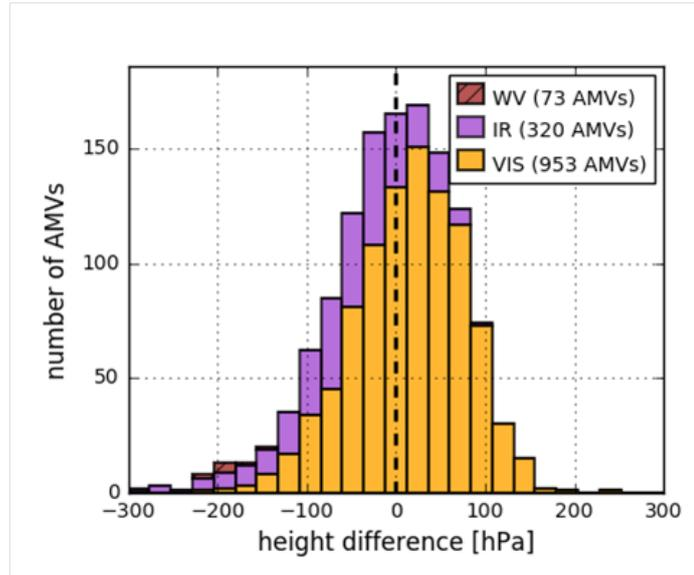
Figure 7: AMV minus lidar height frequency distribution for AMV heights below 700 hPa. Meteosat-10 IR, visible (HRVIS and  $0.8\mu$ ), and WV channel winds in December 2016 with Q11 > 60 and located 20-40N, 0-40E. AMV-lidar matchups are within 50 km in the horizontal and 30 minutes in time..
