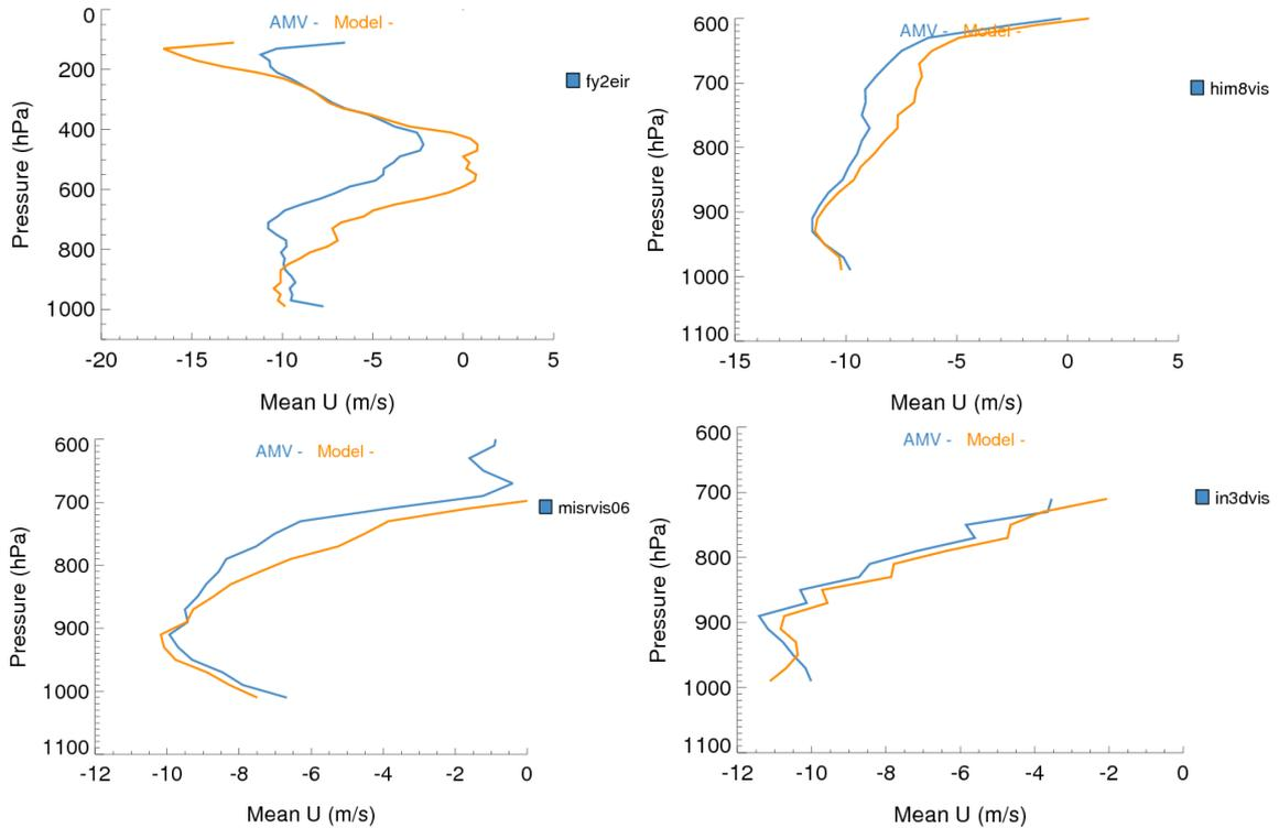
Figure 13: Profiles of mean model and AMV zonal/U wind for FY-2E IR (top left), Himawari-8 visible (top right), MISR (bottom left), and INSAT-3D (bottom right) channels winds. Data for August 2017 filtered for  $QI2 > 80$  (FY-2E and Himawari) or  $QI2 > 60$  (MISR and INSAT) and located between latitude  $25^{\circ} S$ - $5^{\circ} S$ , longitude  $50^{\circ} E$ - $100^{\circ} E$ .
