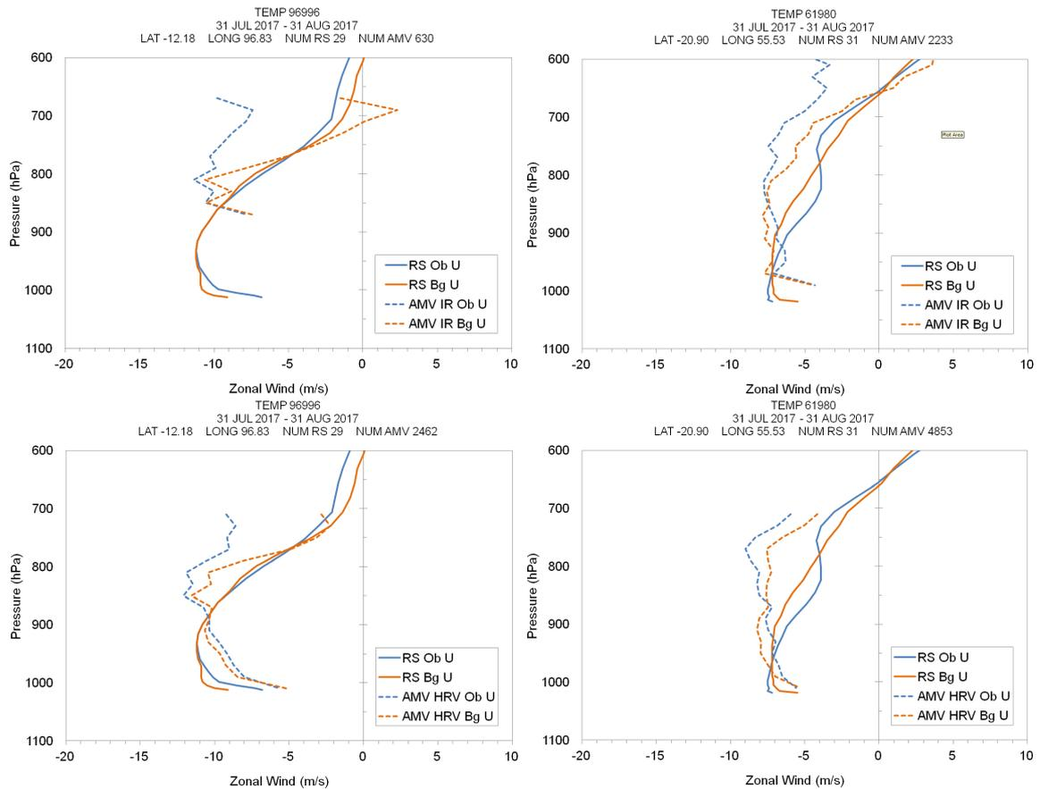
Figure 12: Profiles of mean model background (orange lines) and observed (blue) zonal/U wind component for WMO stations identifiers 96996 (left) and 61980 (right). Data for August 2017. Radiosonde (RS) and RS-background profiles are shown by solid lines, AMV and AMV-background are shown by dashed lines. Meteosat-8 IR10.8 AMVs (top) and high resolution visible (HRV) AMVs (bottom) located in a 2x2 degree box centred on the RS location.
