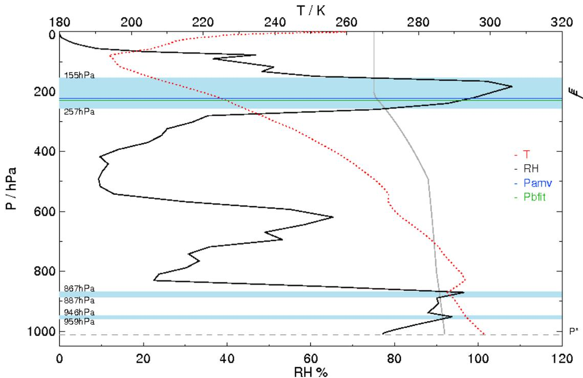
Figure 27: Met Office global model humidity profiles at AMV locations. The top plot shows the AMV's CLA height assignment (blue) and the lower plot shows the OCA height assignment for the same AMV. The model best-fit pressure at this location is shown by the green line. Moist layers (definition from Zhang et al 2010 [2]) are defined by the blue-shaded regions.
