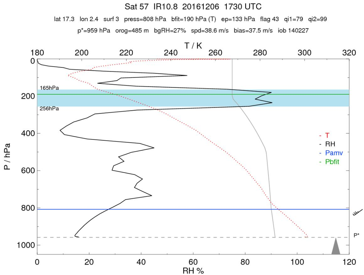
Figure 4: Model profile information for a single AMV extracted at 1730 UTC on 6 December 2016. Model relative humidity (RH, black line), temperature (red dashed line) and surface pressure (grey dashed). AMV pressure (blue line) and best-fit pressure (green line). Blue shading indicates a moist layer where the model RH has exceeded a height-dependent threshold (grey solid line).
