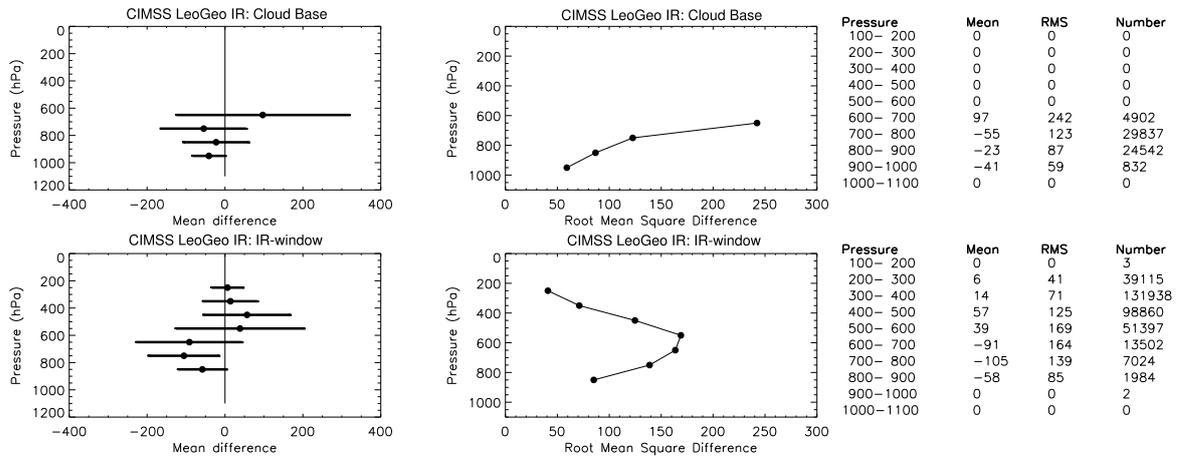
Figure 12: Mean and root-mean square pressure differences of AMVs' assigned pressures compared to their model best-fit pressures, September 2014. Dual-Metop figures are for data polewards of 40° N/S only.
