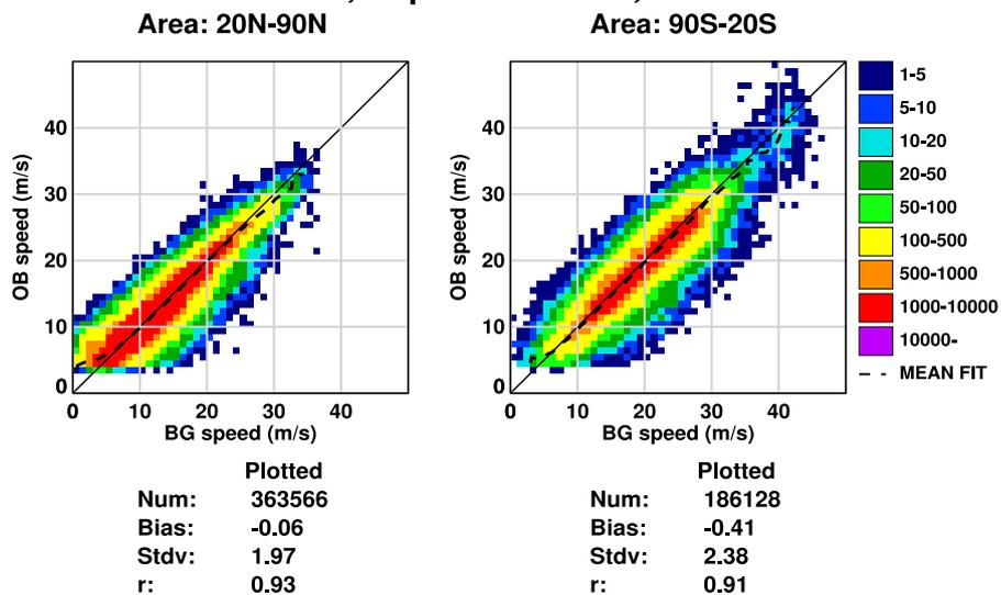
Figure 10: AMV vs model background wind speed for low-level AMVs. Dual-Metop plot is for data polewards of 40° N/S.
