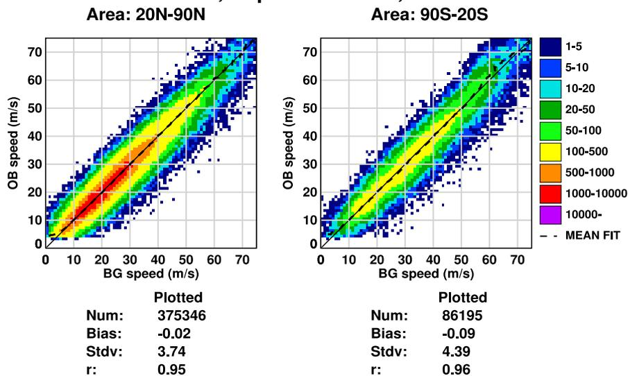
Figure 8: AMV vs model background wind speed for high-level AMVs. Dual-Metop plot is for data polewards of 40° N/S.
