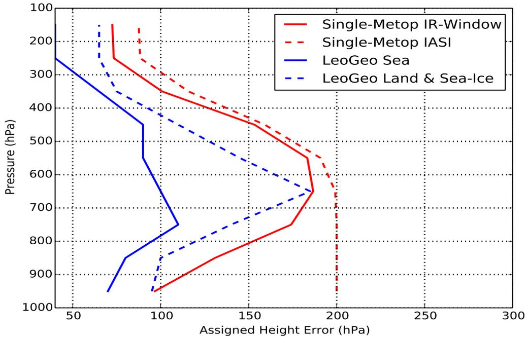
Figure 14: Height error profiles derived from best-fit pressure statistics for the Single-Metop and LeoGeo AMVs. In the Single-Metop trial, 12 separate profiles were used, split by hemisphere, surface type and height assignment method. Averages for each Single-Metop height assignment method are shown here.
