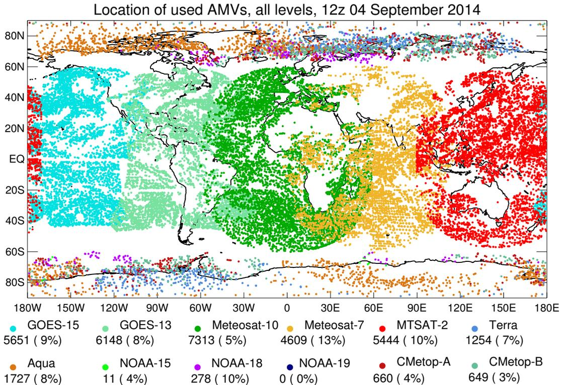
Figure 1: Example coverage of AMVs used in one assimilation cycle of the Met Office global model. There was an outage of NOAA-19 data at the time of the plot. The percentages are the proportions of received data that were assimilated.
